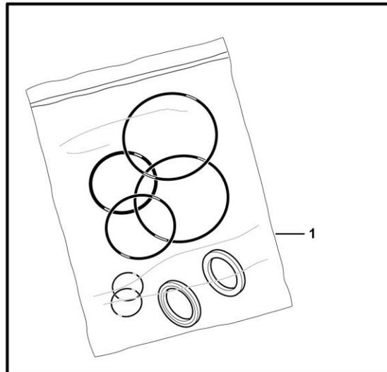
下调平油缸 (10570) Lwr leveling cylinder
