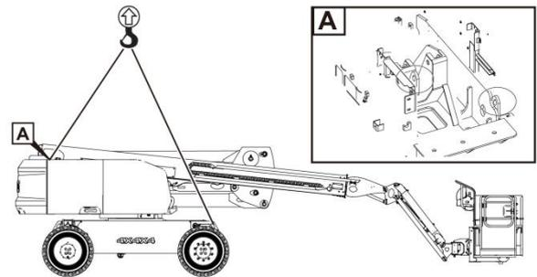
Figure 10-6 Lifting point (take AR20J as an example)
