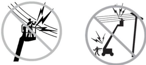
Please maintain an adequate safety distance from electrical wiring, power source and electrical equipment in accordance with applicable laws and regulations and the instructions in the following table.
