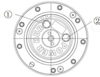
Figure 1-1 Traveling slowdown 1. Oil filler 2. Viewing port
